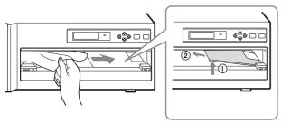
If the tray cover is in the way, remove it by lifting it up 1, and then pulling it out to the direction of arrow 2.
